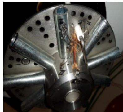
Left: 475 kW burner deck with thermocouples to monitor the temperature. Right: flame image burner
