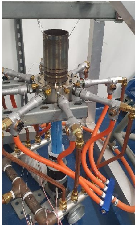
GT combustor set up
